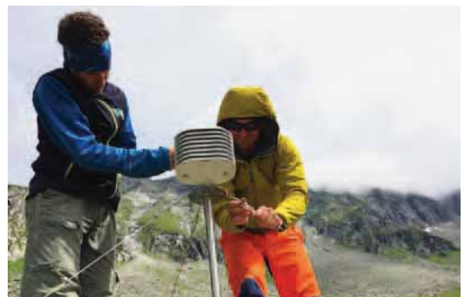
Construction of a weather station near the permanent areas in the Untersulzbachtal valley in the ecological long-term monitoring
