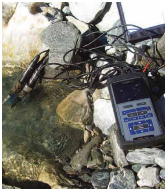
sensor for measurement of chemical parameters of water
